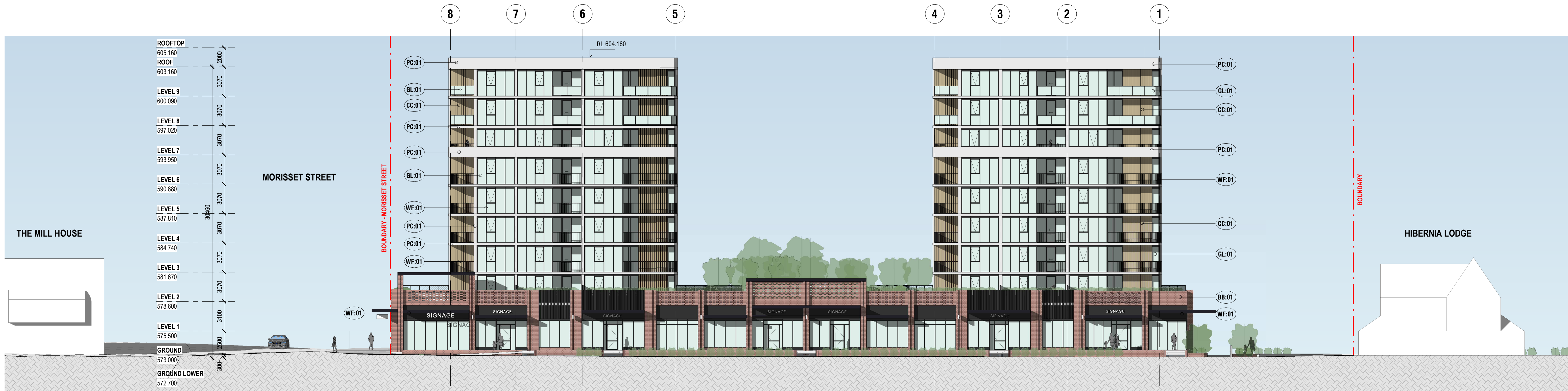
1 EAST ELEVATION - COLLETT STREET SCALE 1:200 @A1
